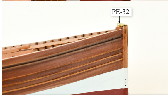
24 - Using a 0.7mm drill bitt, drill a hole for the bow eye-bolt (PE-32) stem, and insert and glue part PE-32 in place.
