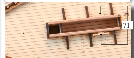
Above - Add part numbers 39, the Fore Mast Opening Side Cheeks. Slot and glue into place as shown above and left. Below - Slot and glue the cleats (71) in place on the outside all of the fore mast housing sides.
