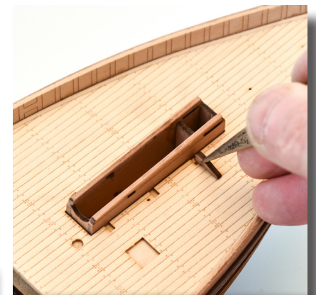
Above - Add part numbers 39, the Fore Mast Opening Side Cheeks. Slot and glue into place as shown above and left. Below - Slot and glue the cleats (71) in place on the outside all of the fore mast housing sides.
