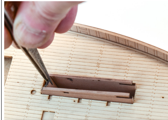
Above - Slot and glue part number 34 into the rear of the fore mast structure.
